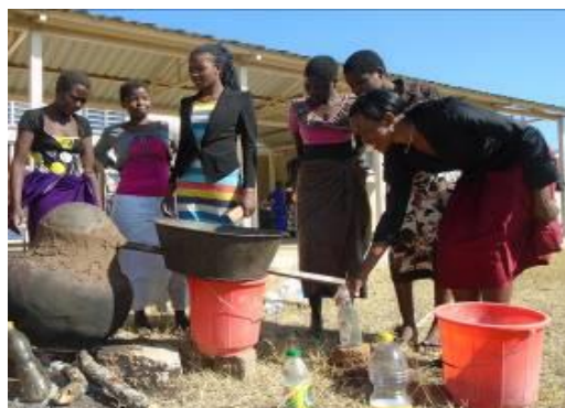
Fig 3.3: Traditional distillation apparatus used to separate mixtures
