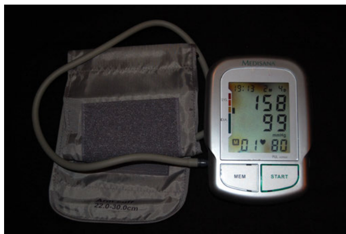
Figure 8.22: The instrument used to measure blood pressure is a sphygmomanometer . This figure shows an automated arm blood pressure meter showing arterial hypertension. From the top reading systolic pressure is 158 mm Hg and diastolic reading is 99 mm Hg and the heart rate is 80 beats per minute.
