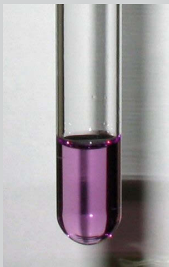
Figure 2.18: Biuret test: this is the expected colour change if protein is present
